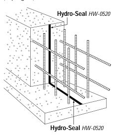
Vertical 90° corners, vertical "T"s and vertical "X"s should be butted and bonded with cyanacrylate adhesive.
